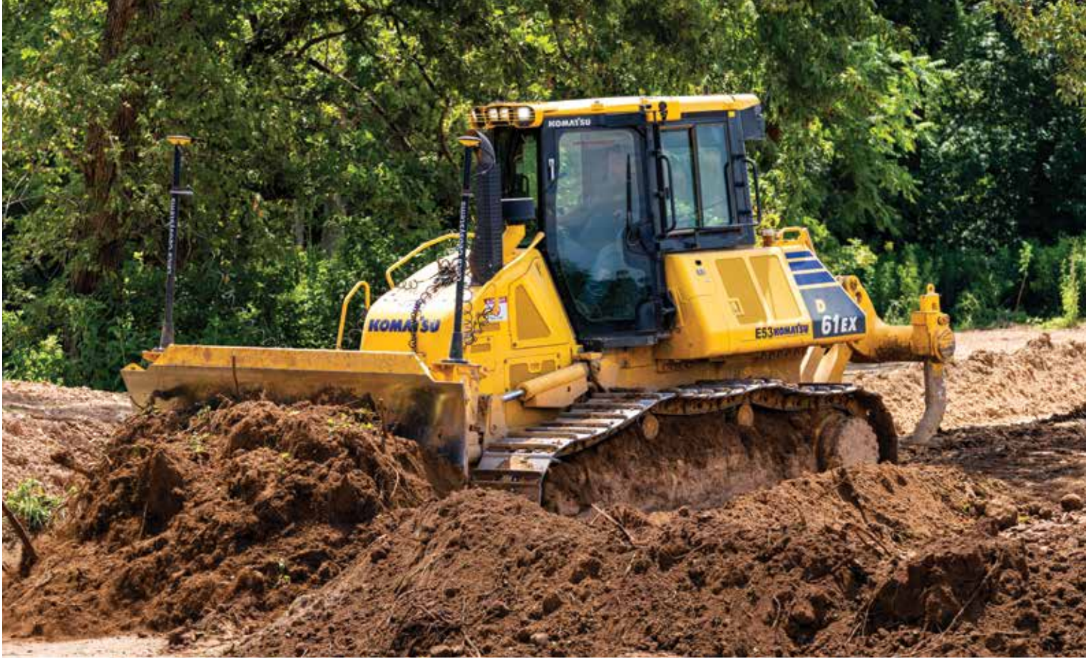
An operator pushes out a pile of dirt with a Komatsu D61EX dozer.
