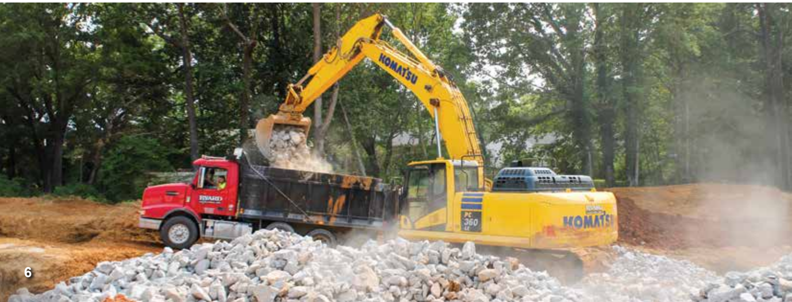
An operator loads stone into the bed of a truck with a Komatsu PC360LC excavator.
