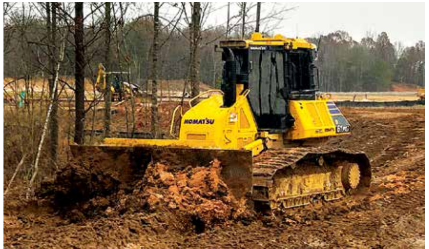
An operator uses a Komatsu D61PXi-24 intelligent machine control (IMC) dozer.
