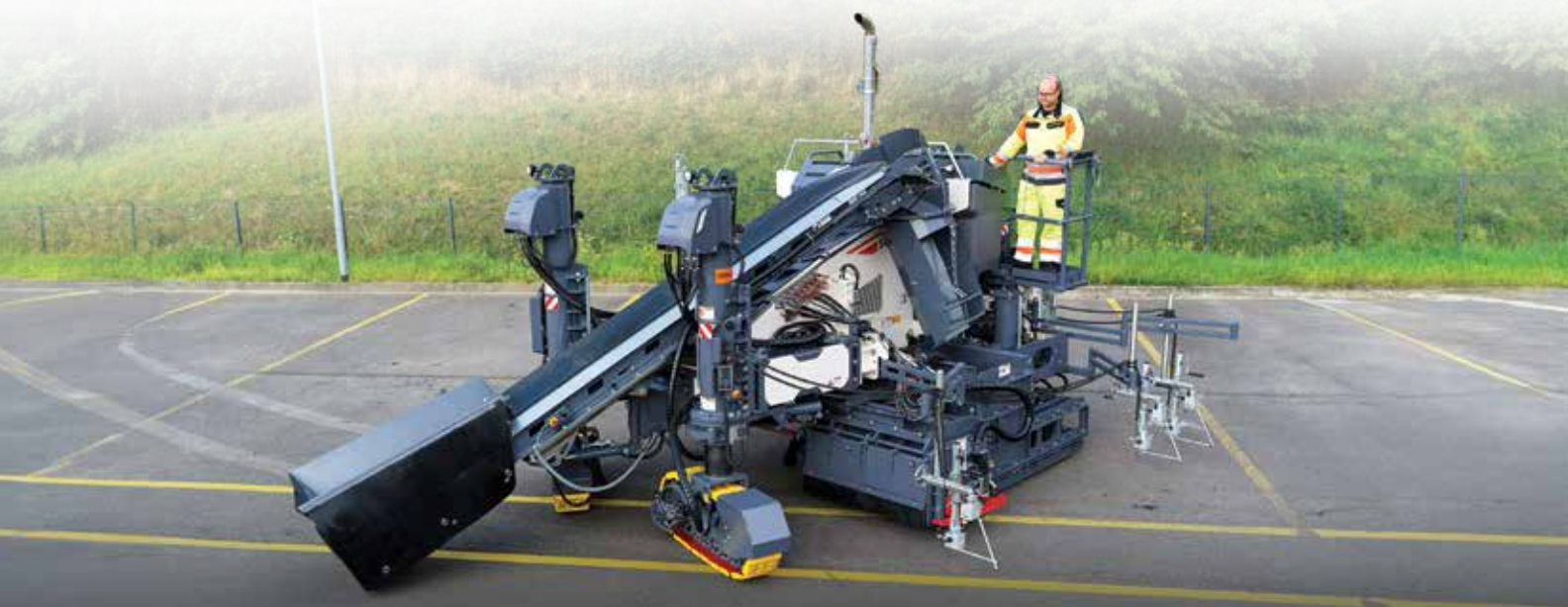
WIRTGEN's new SP 33 slipform paver can pave concrete slabs up to 7 feet wide in the offset paving configuration and up to 10 feet transversely to the direction of travel.
